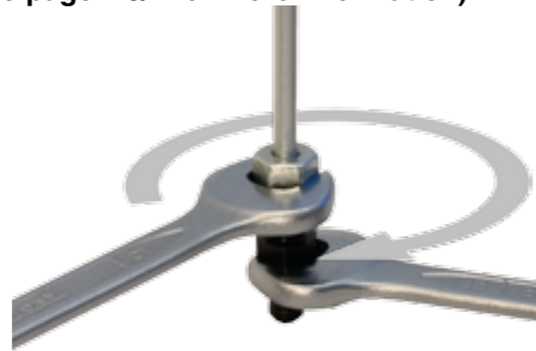
2. Then tighten until sharp increase of resistance approximately 1 turn (if possible use torque according to next page)
