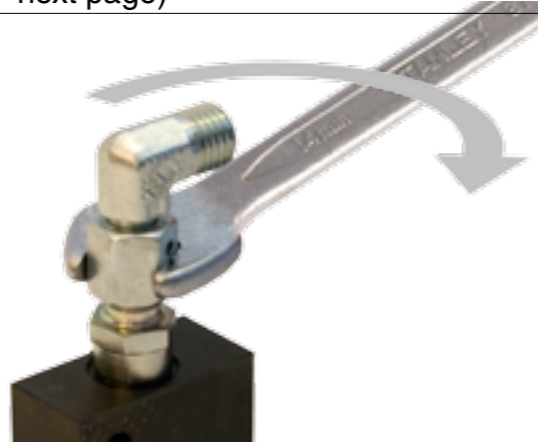
2. Then tighten until sharp increase of resistance ¼ to ½ turn (if possible use torque according to next page)
