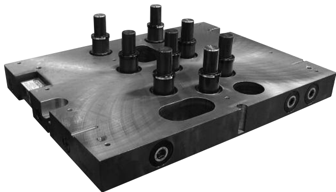
Standard manifold with clearances for die details.
