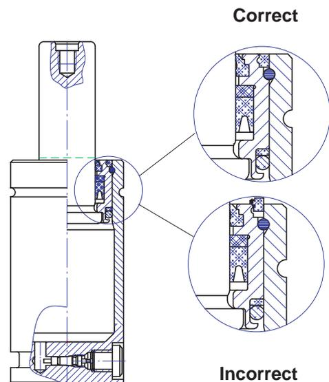
The function of the dirt protection ring is to prevent dirt from penetrating into the gas spring and also prevent the guide from falling into the tube when the spring is uncharged.
