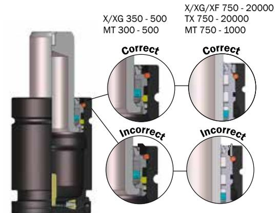
The function of the dirt protection ring is to prevent dirt from penetrating into the gas spring and also prevent the guide from falling into the tube when the spring is uncharged.
