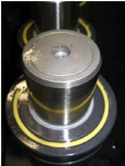
Example of a present combination of identification grooves on a TU 5000 spring.
