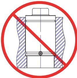
Never mount a gas spring in a pocket that does not fully support its base
