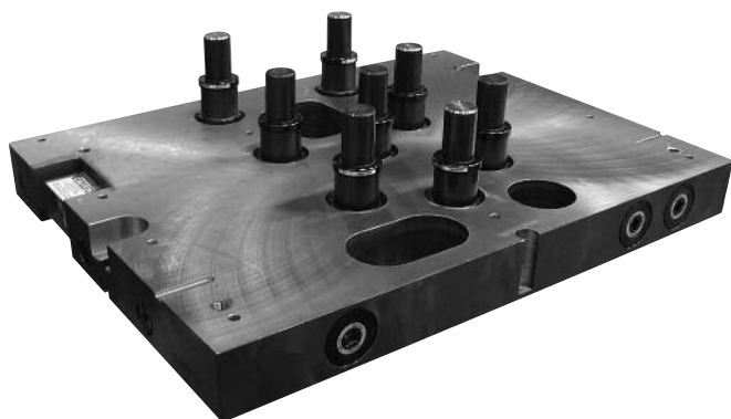
Standard manifold with clearances for die details.
